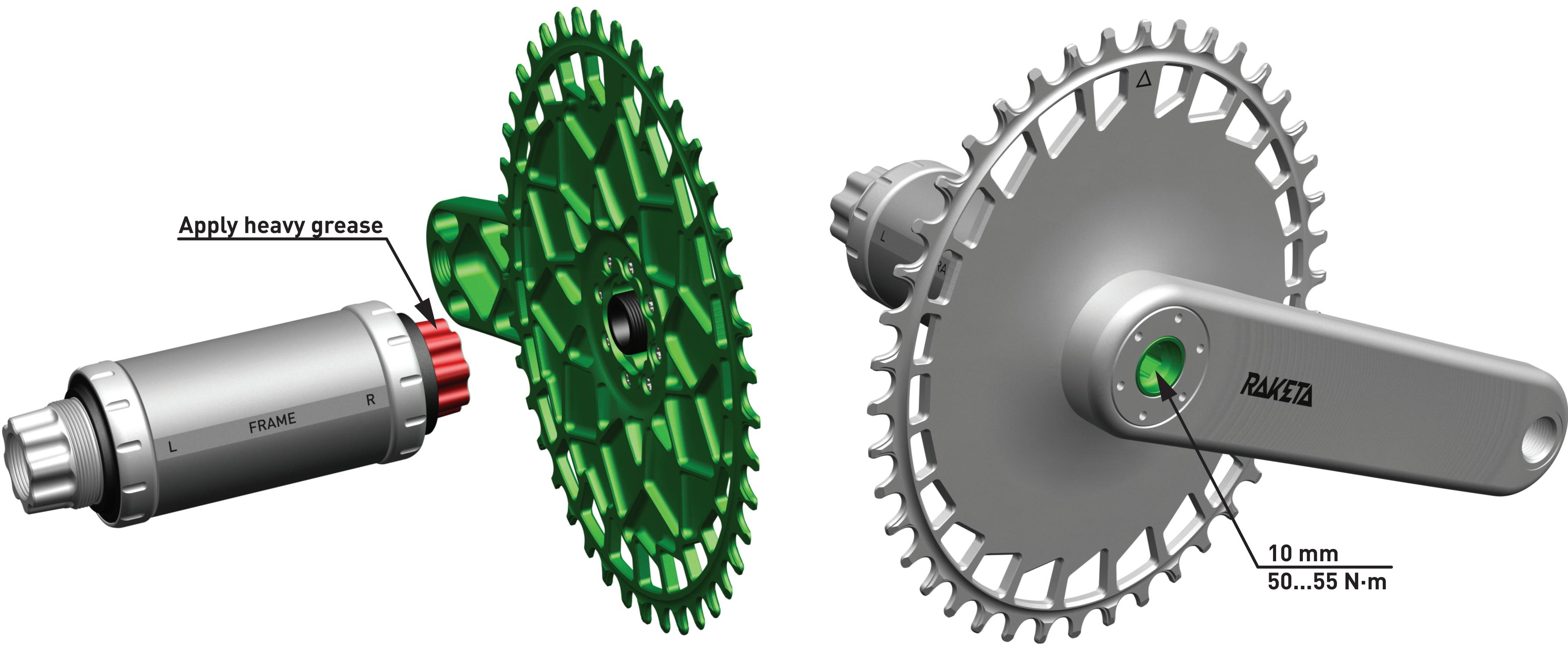
Apply heavy grease (like bearing grease) to the splines of the axle and install the right crank arm. Use a torque wrench with a 10 mm hex bit socket to tighten the crank arm bolt to 50...55 N·m. Make sure to align the splines on the crank arm and on the axle during installation.
