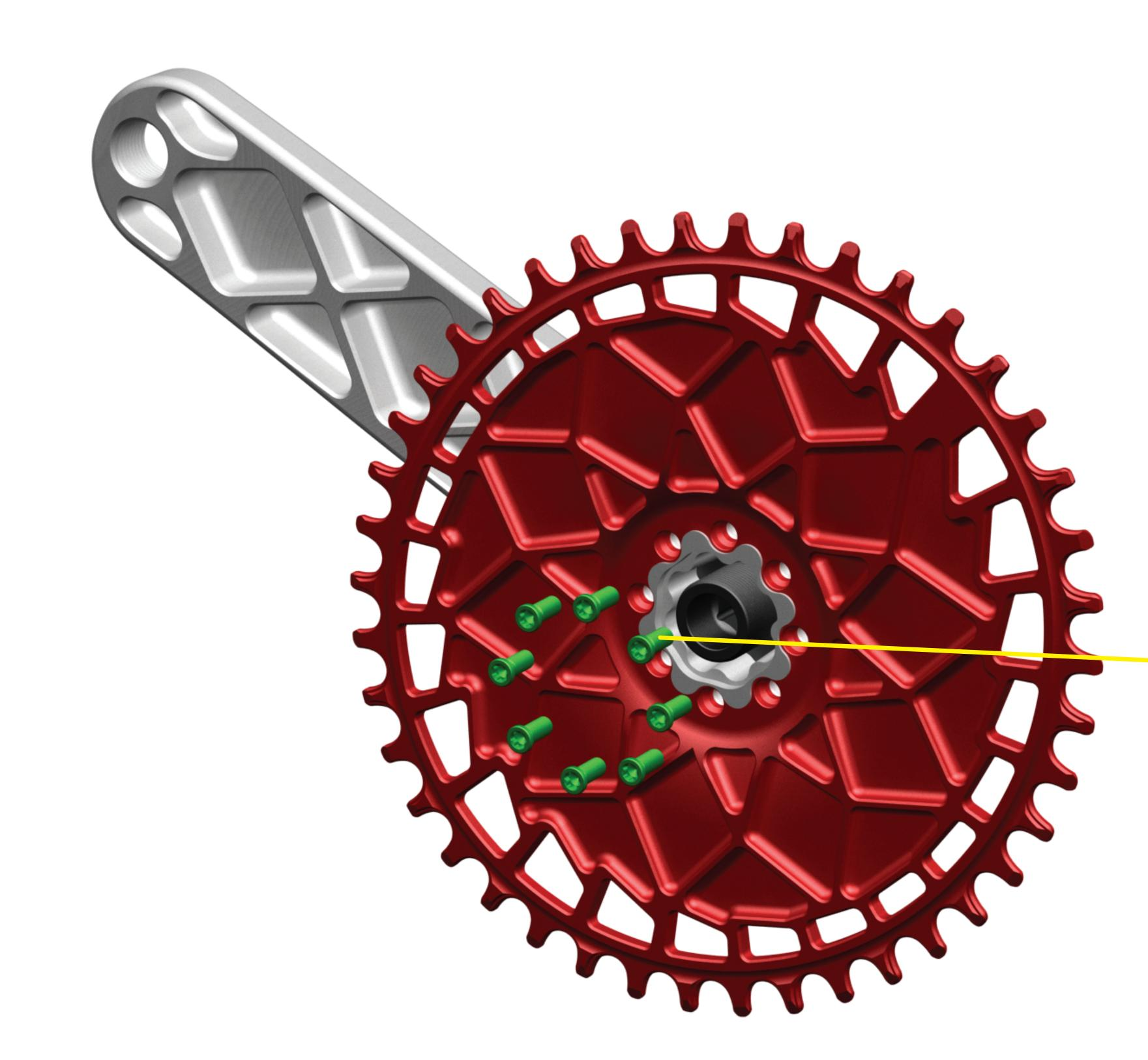
Install the chainring (spider) onto the drive side crank arm with the mounting bolts. Note that there is only one possible position for the chainring (spider).
